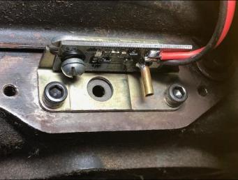
Install the sub-assembly on the engine using the supplied socket-head fasteners & internal star washers
