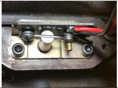
Slide the torsion spring over the pivot-shaft; Deflect as required to clear the socket-head and mate with the slot
