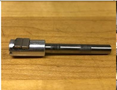
Install the magnetic head on to the OEM push-rod as shown above
