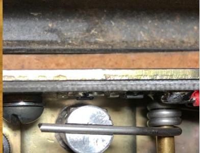
Install the magnetic head assembly in place; Note that the magnets MUST face the KHET PCB
