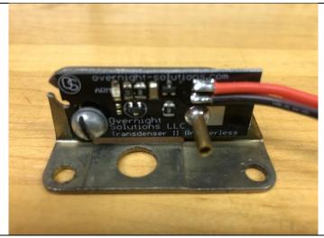
Remove OEM breaker-points from breaker-point bracket & install the KHET switch module
