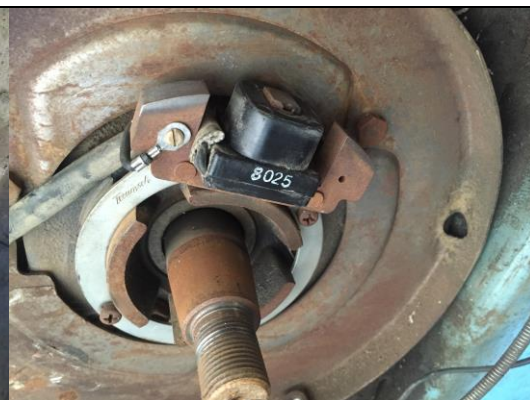
610965 Charge Coil NLA BUT I rebuild them (Inductance test only)
